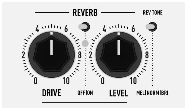
This amplifier is equipped with an analog spring reverb. A powerful 12BH7 tube drives a three-spring reverb tank with a medium decay time of two to three seconds, depending on the signal strength. The reverb signal is fed directly back into the phase inverter of the power amplifier, where it is mixed with the dry guitar signal.
