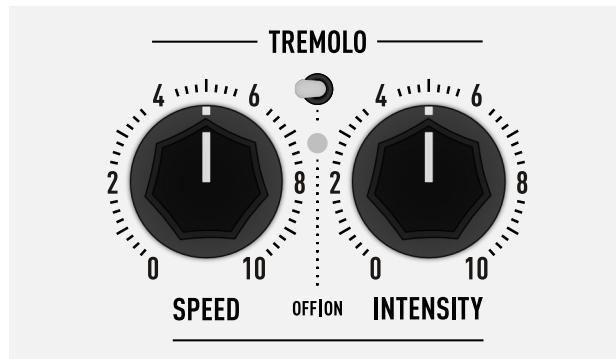
Excelsior Deluxe features a tube driven tremolo effect by modulating the bias voltage of the power amp tubes. The modulation looks more like a sine wave, resulting in a soft or vintage characteristic.
